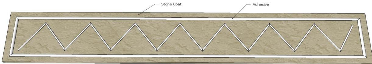
4. You may need to use temporary mechanical fasteners to secure the moulding in place while the adhesive cures. For example: galvanized nails or screws and washers. You can also use oval top nails fixed into the wall then simply push the profile onto the nails. These hold the profile in place while the adhesive cures and they do not require removing.
